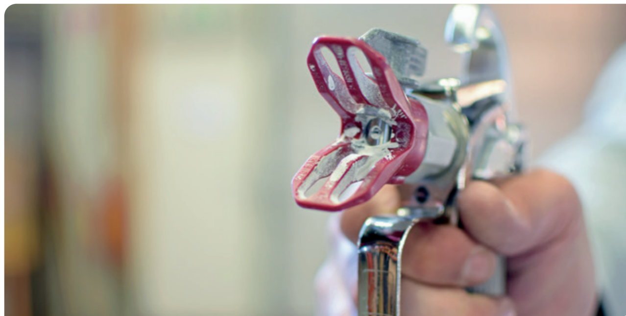
Figure 8a: Airless spray gun
