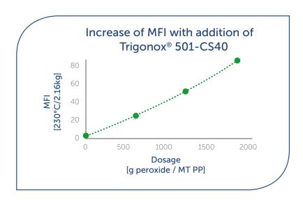
Trigonox® 501-CS40 is superior to traditional vis-breaking peroxides; in fact, it shows a 60% reduction in the Volatiles Organic Compounds produced during extrusion and can be stored at room temperature.
