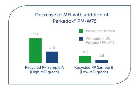
With the use of Perkadox® PM-W75 the melt strength and melt elasticity of the modified recycled PP increases strongly, enabling new processing opportunities and applications like foaming, blow molding and even thermoforming.
