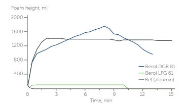
Foaming profile of Berol DGR 81 and Berol LFG 61 when tested in the circulation method. Albumin was used as foaming agent. The graph shows that Berol LFG 61 provides anti-foaming properties in this system.
