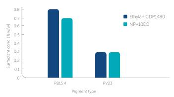
Amount of surfactant needed for wetting 2.5 wt% pigment in aqueous solution. Comparison of Ethylan CDP1480 with standard nonionic surfactant NP+10 EO
